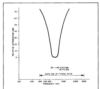
fig. 4. CW filter attenuation response is shown in a semi-log plot relative to the audio bandwidth of a typical Amateur receiver. About 75 percent of the undesired audio bandwidth is attenuated 30 dB or more.
